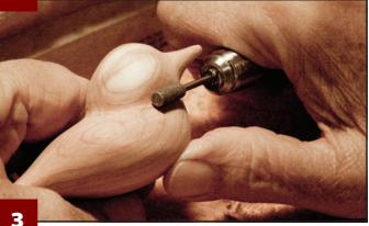
**Finish shaping the bird.** Use a carving knife to shape the beak. Use a rotary-power carver and your bit of choice to add any desired details and to remove any remaining ridges. Make sure the bird is smooth and flowing with no hard lines or sharp angles.
