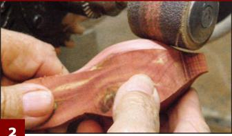
Rough out the bird. Remove the sharp edges and rough shape the bird with a sanding drum equipped with 60-grit sandpaper. I use a 1½" (38mm)-diameter drum attached to a radial arm saw, but you can use a rotary-power carver. Shape the neck with a 1" (25mm)-diameter cushioned sanding drum.
