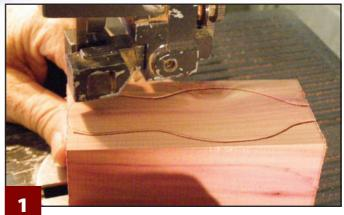
**Cut away the excess wood.** Create templates by transferring the patterns to thin cardboard and cutting around the outline of the patterns. Trace the templates onto the blank and cut the top view of the bird with a band saw. Tape the waste in place, rotate the blank 90°, and cut the side view.
